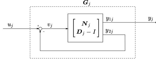
**Fig. 2.** Coprime factorization as a coupled system.
