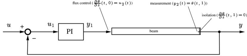
**Fig. 3.** A heated beam with a PI-controller.
