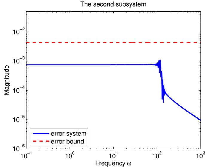
**Fig. 7.** Example 2: the absolute error  $\|\tilde{\mathcal{G}}_2(i\omega) - \mathcal{G}_2(i\omega)\|_2$  and the error bound  $\gamma$ .
