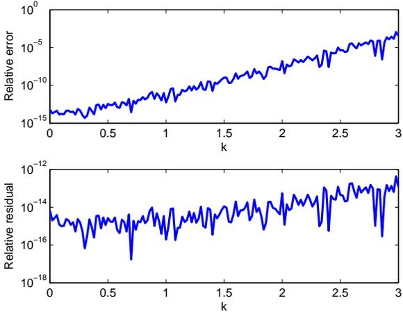
Fig. 2. Relative errors (top) and relative residuals (bottom) for the projected continuous-time Lyapunov equation.
