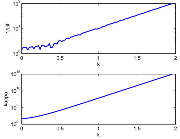
Fig. 3. Reciprocal of the separation  $\text{dif} = \text{Dif}$  (top) and the condition number  $\kappa = \kappa_d(E, A)$  (bottom) for the projected discrete-time Lyapunov equation.
